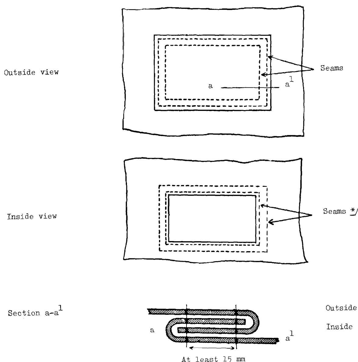
\*/ Threads visible from the inside shall be of a colour different from that of the threads visible from the outside and from that of the sheet.
