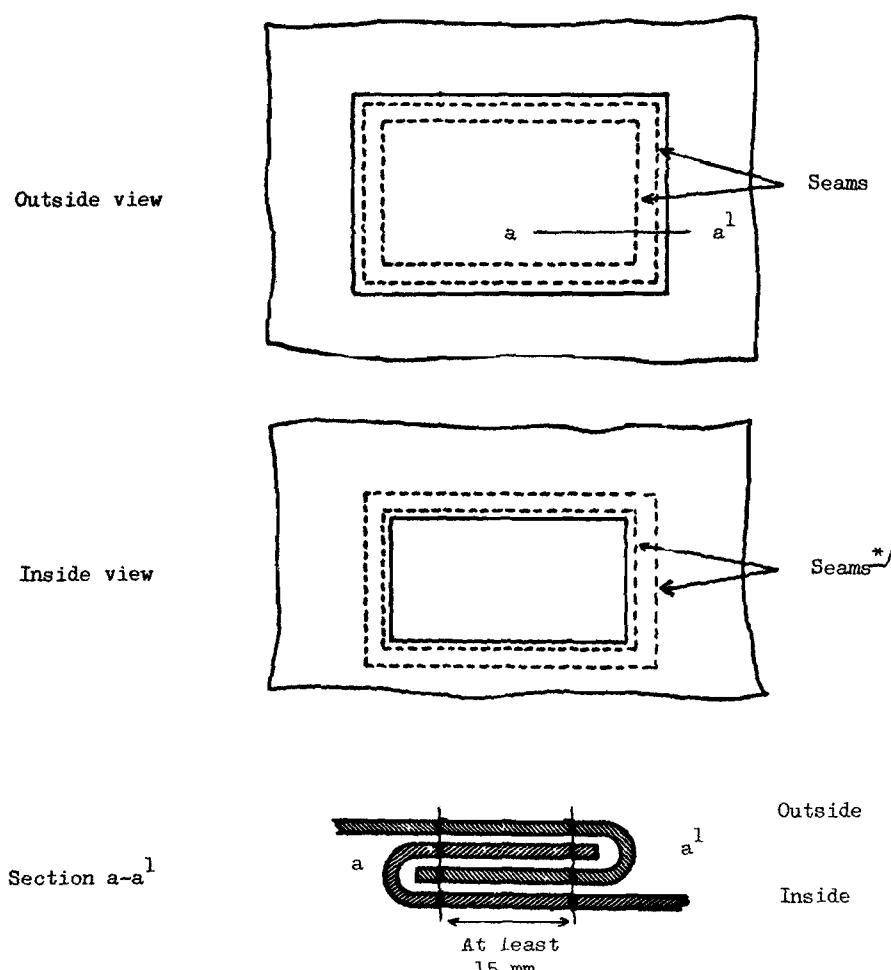
\*/ Threads visible from inside shall be of a colour different from that of the threads visible from the outside and from that of the sheet.
